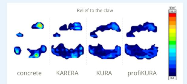
Pressure measurements carried out on bovine claws by the Leipzig University: reduced pressure peaks through use of rubber (rather than concrete), leading to better pressure distribution – more similar to pasture ground.
