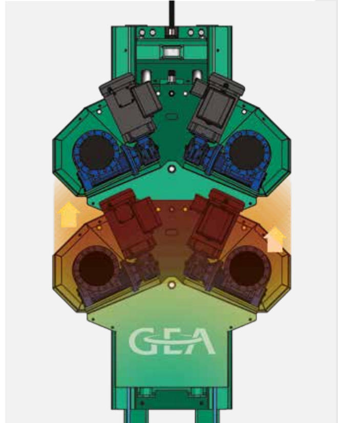
The Fit R-300 drive unit moves one side upward after the other, along the two guide pillars, until it reaches the end of its stroke.
