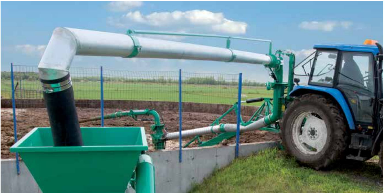
Articulated Loading Pipe installed on an Articulated Agi-Pompe
