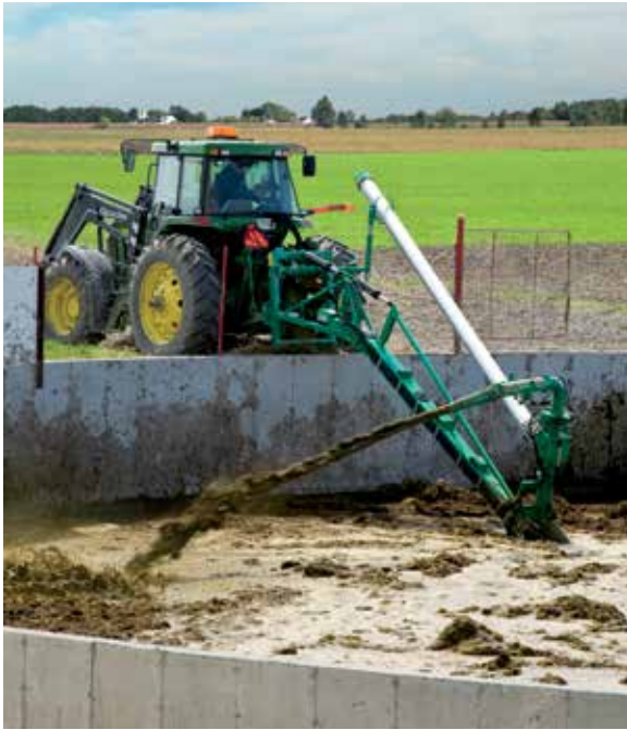
Articulated Agi-Pompe with the optional articulated housing
