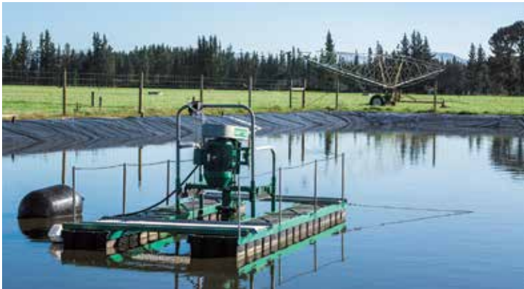
8" flush pump on 12-ft. (3.7 m) pontoon with six floats. A 16-ft. (4.9 m) pontoon with eight floats is also available for the 50-HP (37 kW) and larger motors.
