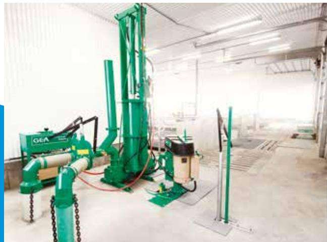
Electromix system on the floor above the reception pit. Installation with double discharge for manure transfer in two different pits.
