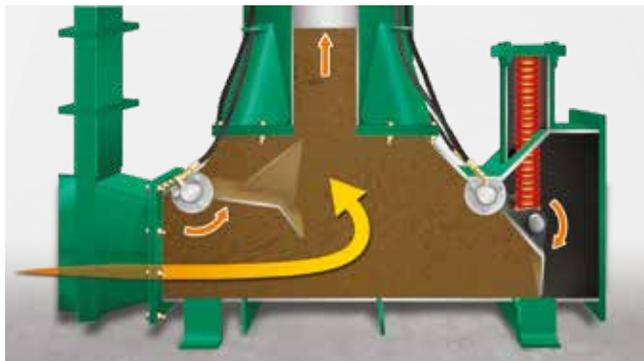
During the evacuation cycle the pressure exerted by the piston downstroke closes the intake valve and forces the discharge valve to open, allowing evacuation of manure. The downstroke lever attached to the intake valve ensures complete closure of the pump inlet.
