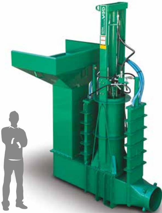
Several types of hoppers are available for installations comprising 1 or 2 barn cleaners, or for skid-steer loader scraped alleys in free stall barns. The pump hopper can be replaced by a suction pipe and reception pit if the manure does not contain bedding.
