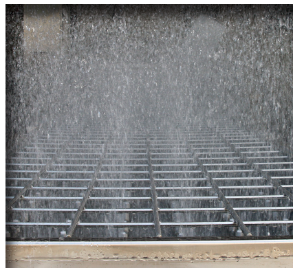
Cone spray nozzles for clean spray and excellent bottle coverage.
