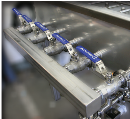
Individual valve zone control for washing at less than full capacity.
