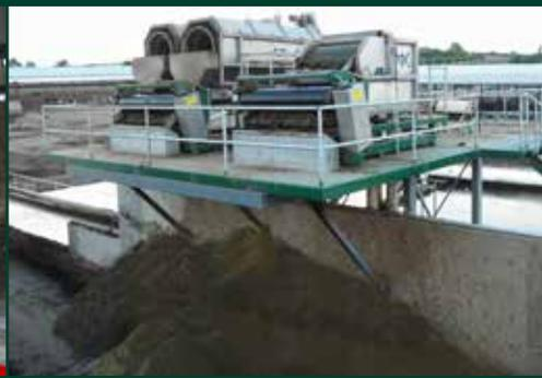
With the introduction of the wedge wire screens in all model sizes, each model can be configured for standard separation, bedding or high capture separation. With high capture separation, a fine screen can be used for closed loop flush, flush flume systems, secondary separation, or high capture primary separation.
