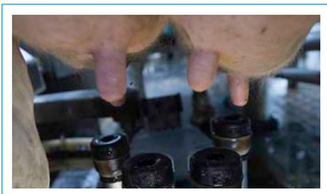
GEA robots are equipped with patented and legendary **StimoPuls technology**—a mechanical stimulation system backed by decades of use with GEA pulsators on conventional parlors. StimoPuls stimulation begins as soon as the teat cup attaches, at the same time as cleaning in an ideally timed sequence.
