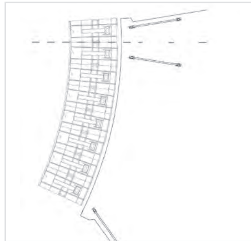
V-Shaped entrance: Allows a cow to enter the platform while the second cow establishes position. This configuration must be used with PPID (per place individual ID) systems.
