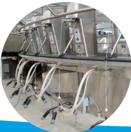
PosiForm Drop-down Hose Support - drops units below the deck when not milking and out of the way of the operator.
