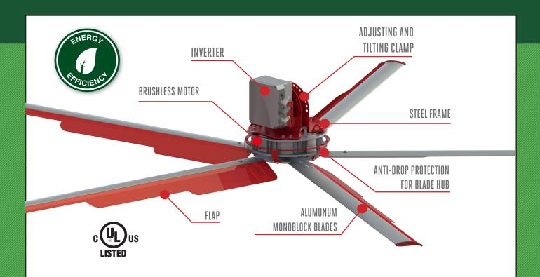
ZEFIRO fans are the flagship product of CMP. The main characteristic of this product is the brushless motor, which employs an onboard mechanism to regulate the speed automatically. This innovation removes the gear box present in traditional asynchronous motors, which reduces the presence of mechanical parts subject to wear. This innovation results in less maintenance, more efficiency and less energy consumption.
