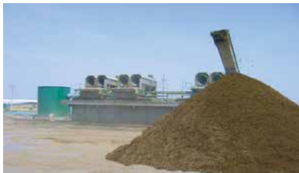
Primary and Secondary separators with upflow sand sedimentation tank on Biolyнк system handling flush manure from 8,000 cows in freestalls in Eastern Oregon.
